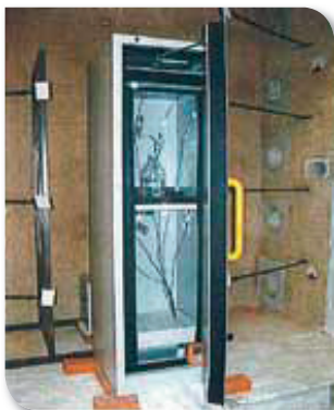
Exacta cabinet series EFO BEFORE fire resistance test.
