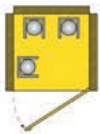
K89052 - LED3 For 3 gas cylinders W960 x D880 x H2400mm Weight: 262 Kg
