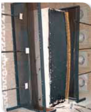
Exacta cabinet series EFO AFTER fire resistance test.
